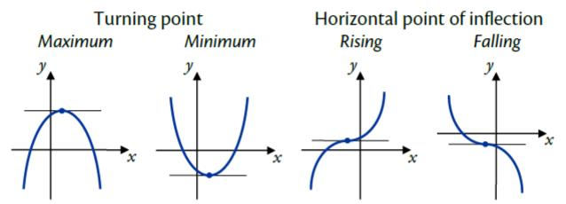
A stationary point's nature (type) is determined by the behaviour of the graph to its left and right. This is often done using a "nature table".
